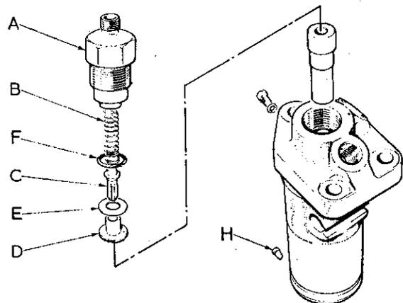
3. Remove the top nipple (A) on the fuel injection pump. Then remove the delivery valve spring (B) & delivery valve (C).
