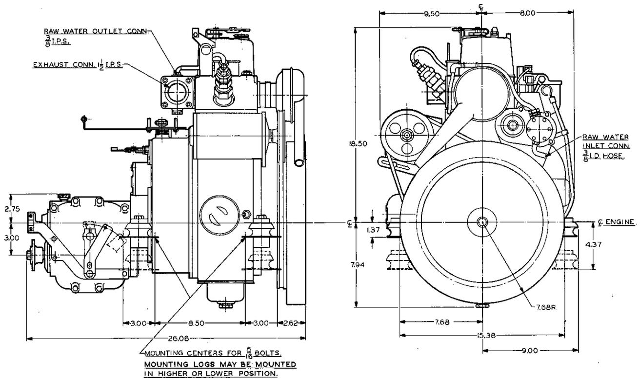
Fig. 26 Measurements of PILOT 10
