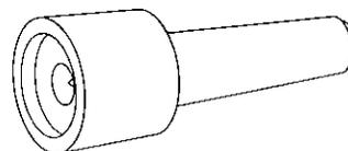
TOOL FOR PRESSING IN CAMSHAFT BEARING
