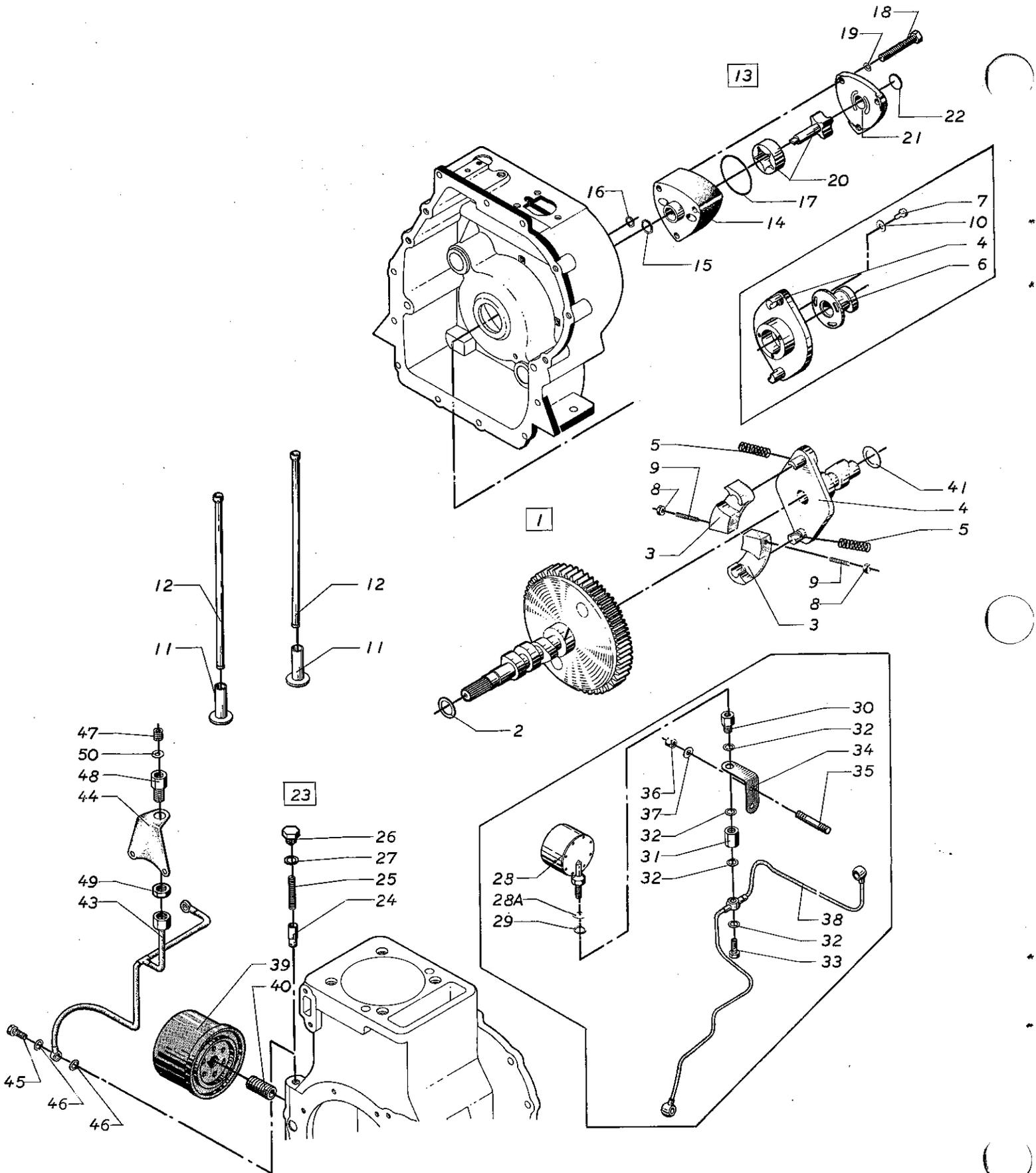
WESTERBEKE 10: CAMSHAFT - LUBE OIL PUMP AND FILTER
