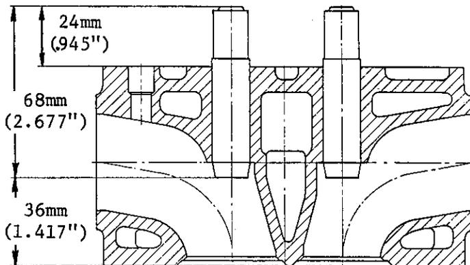
Dimensions for replacing valve guides
