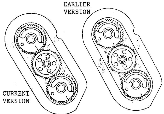
MARKS ON COUNTERWEIGHTS AND CRANK GEAR
