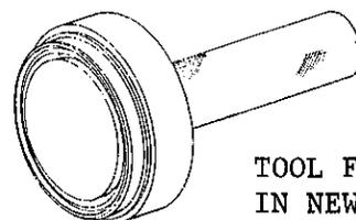
TOOL FOR PRESSING IN NEW OIL SEAL
