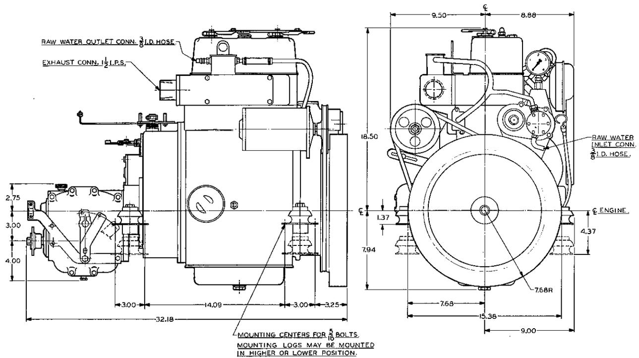
Fig. 27 Measurements of PILOT 20
