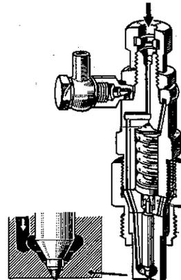
Fig. 18 Injection nozzle
