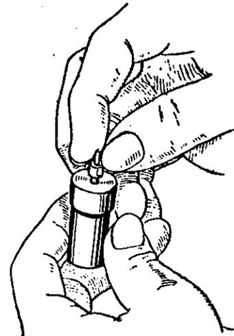
After examining the external appearance of the nozzle, the following test should be carried out: The needle should be dipped in diesel fuel and lightly inserted in the nozzle body. As soon as the needle has entered its bore it should drop into its seat easily, without any resistance. The final test for making sure that the needle is functioning properly is to pull the needle up one third of its total length then release it. The needle should drop onto the seat in the body by its own weight.
