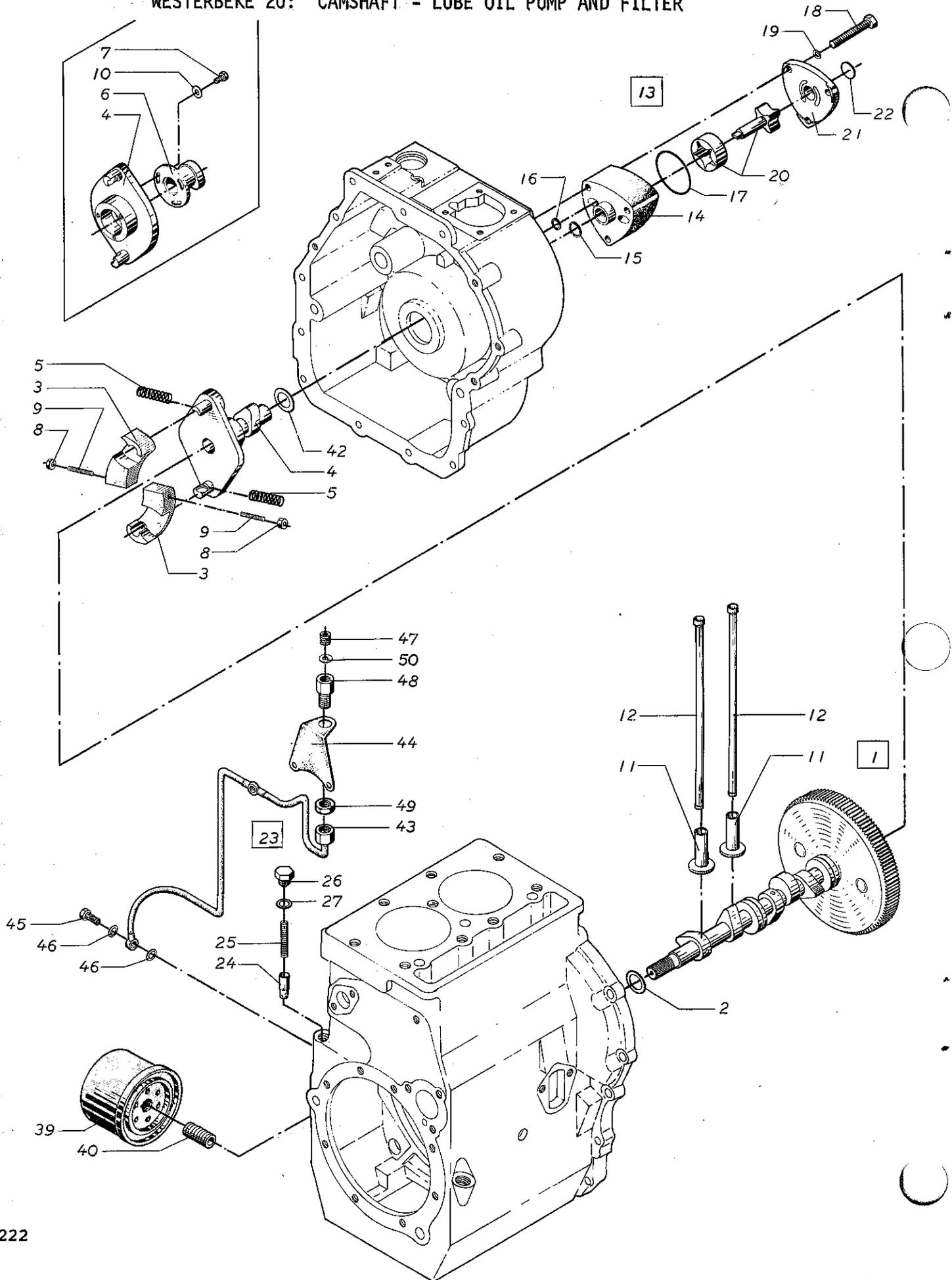
WESTERBEKE 20: CAMSHAFT - LUBE OIL PUMP AND FILTER
