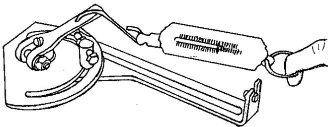
1. The tightness of the governor arm may be adjusted by changing the number of teller springs (4). It is important that the tightness of the arm is adjusted to suit remote or direct operation. If remote controls are used set the adjustment to 4.5 kg (9.9 lbs.). This overcomes friction in the cables as well as the remote control box. For direct operation, set adjustment with a torque of 6 kg. (13 lbs.).
