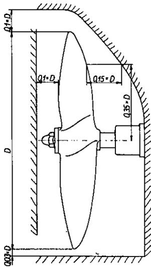
Fig. 31 Clearance of propeller (minimum)
